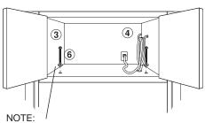
Screw length has been designed to accommodate 3/8" and above cabinet depth. If less, screw must be cut to required length.
